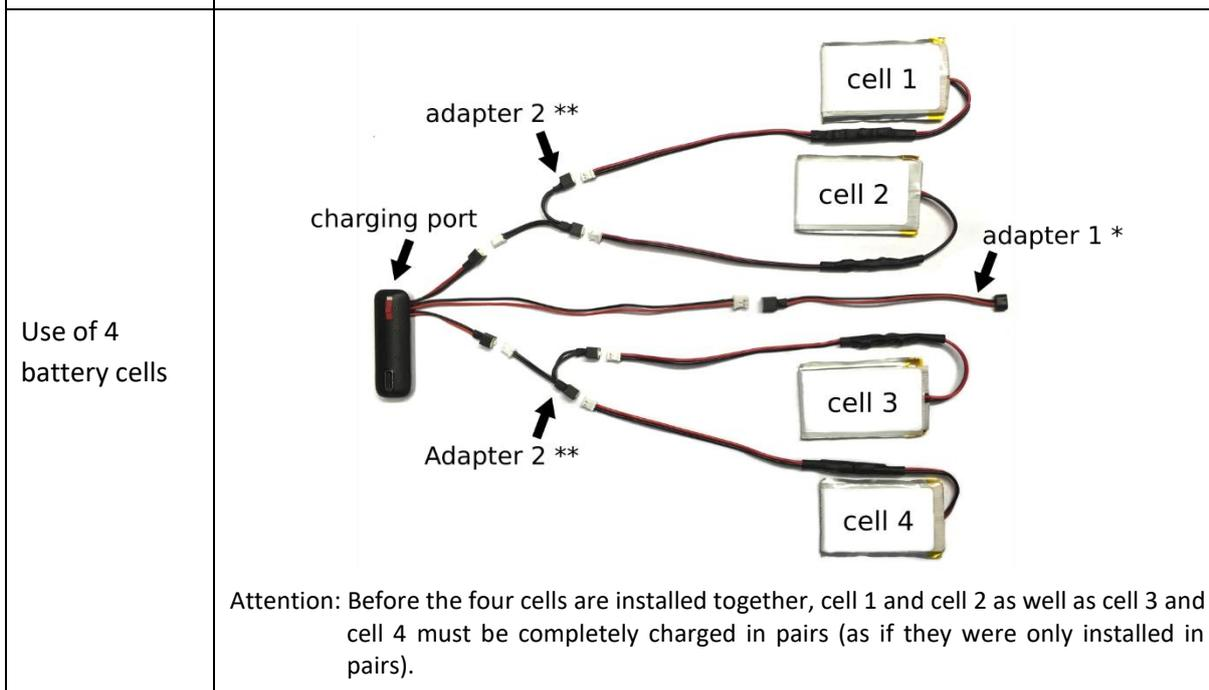
\* Adapter 1: Adapter cable between charging port and coaxial connector, required for *VINCENTevolution* and *VINCENTyoung*, for the *VINCENTpartial* not required.
